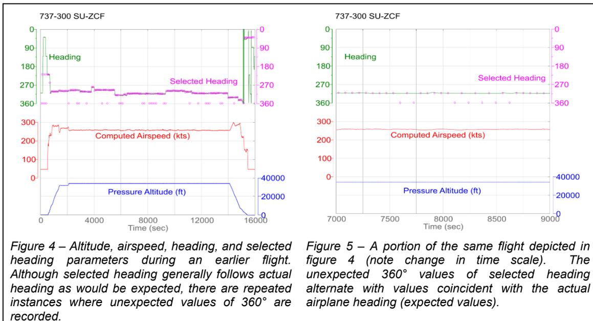
A common practice among DFDAU manufacturers is to use alternating patterns to indicate errors in the FDR data. For example, “stale data”, occurs when a source stops transmitting data to the DFDAU or the transmitted data is not received by the DFDAU. Consultation with the manufacturer of the DFDAU confirmed that the
