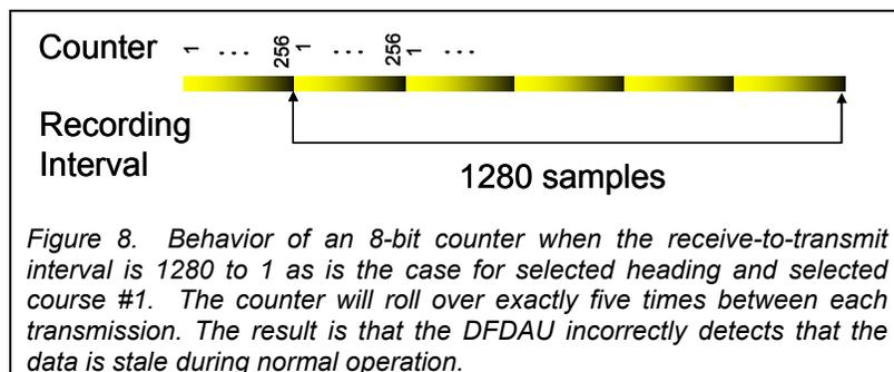
are transmitted to the FDR. If the parameter value has not changed, the DFDAU will incorrectly detect that the data is stale, even though the correct number of samples (1280) has been received.
