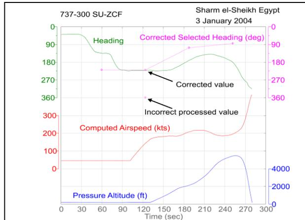
Figure 9 – The same data as depicted in figure 1 corrected to account for the anomaly discovered in the way the DFDAU processed the selected heading data. This was the data used for the analysis portion of the investigation.
