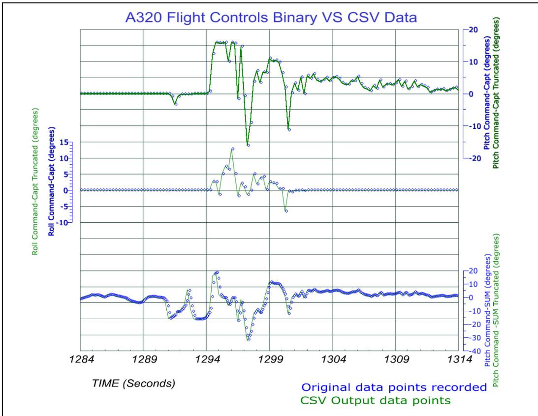
Figure 12 – Comparison of A320 side stick position data recorded at 4 Hz. The original binary data points are shown as blue circles. The same data processed by the CSV method is shown as green lines. Note the time shift as the CSV method positions the 4 Hz data to the nearest ¼ second rather than at the actual time recorded.
