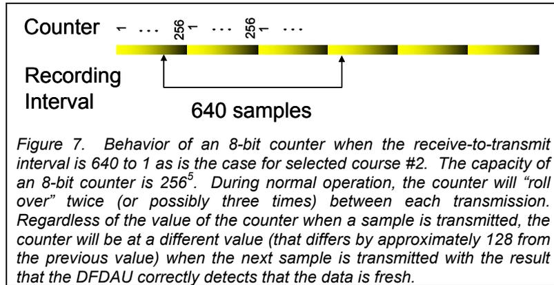
FDR. Regardless of the value of the counter when a sample is transmitted, the counter will be at a different value (that differs by approximately 128 from the previous value) when the next sample is transmitted. The result is that the DFDAU can correctly determine if the data is fresh or stale.
