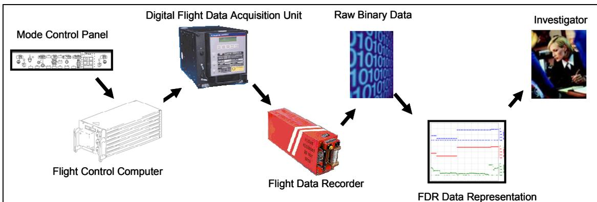
Figure 2 – A graphical depiction of the provenance of the selected heading parameter recorded on a 737-300 FDR. The data originates in the mode control panel and passes through a number of distinct transformations before being utilized during an investigation.
