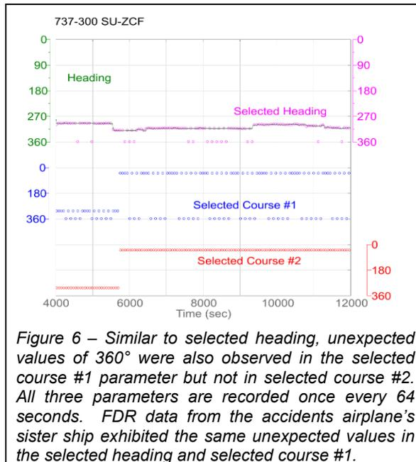
Accordingly, the inquiry focused on how the DFDAU detected stale data. According to the DFDAU manufacturer, stale data is detected as follows:
